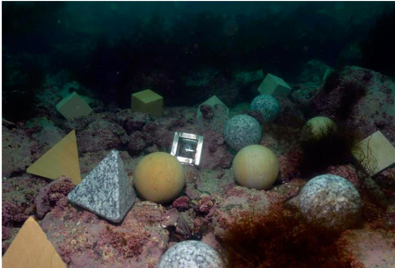
Fig.2. Study investigating influence of substrate dynamics on biota colonization. Machined rocks of different shapes, each shape representing different dynamics of substrate. The metal cube frame has a mounted movement logger inside.
