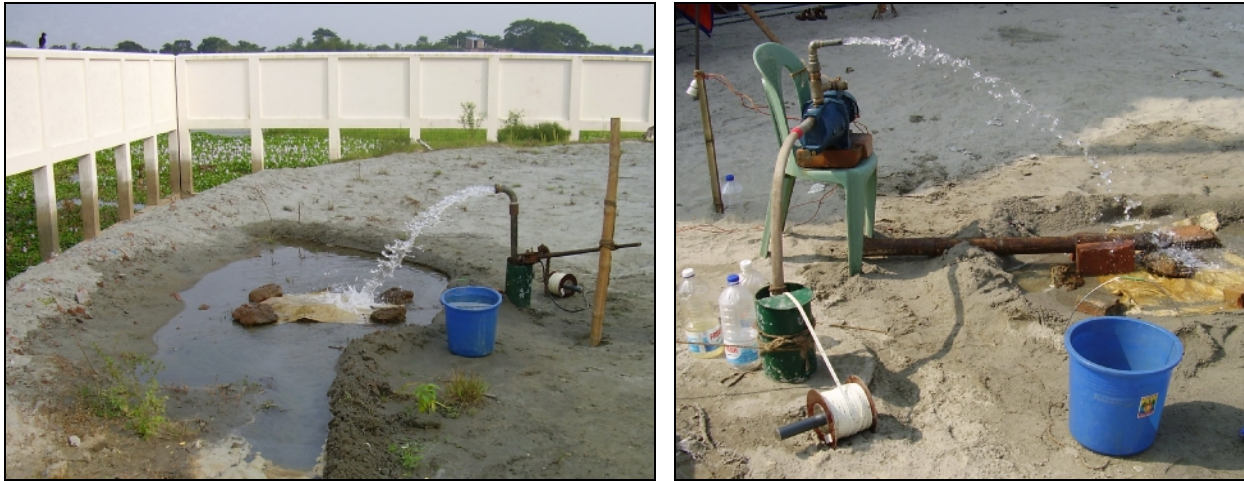
Figure 17 Pumping tests at the test site, using a submersible pump at the 280 ft well (left picture) and a suction pump at the 85 ft well (right picture). (The left picture shows that the agricultural low-land besides the test site partly still is inundated and overgrown by floating water hyacinths in beginning of November 2007)
