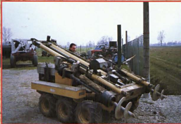
PENETROMETER TG 73-200 kN SELF-ANCHORING SYSTEM STATIC-DYNAMIC- ROTARY 6x6 SELF-PROPELLED
