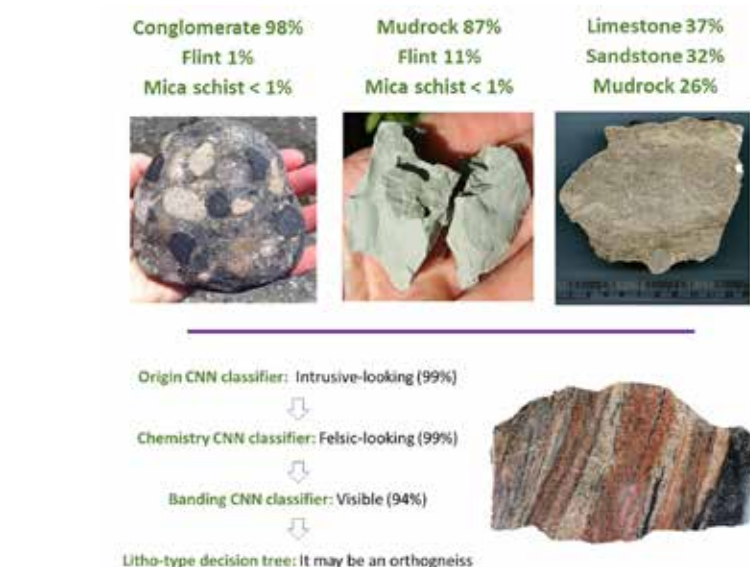
Figure 4: Automated identification of lithofacies on field samples with artificial intelligence algorithms. Top: direct lithology classification. Each input picture displays the three most probable classes according to the neural network. The first two pictures are archetypal and the probabilities neatly favour a single class. However, the third picture is more ambiguous and the probabilities reflect the uncertainty that a human geologist would face. Bottom: lithology classification combining petrological feature recognition and a decision tree. Adapted from Bouziat et al. 2020.
