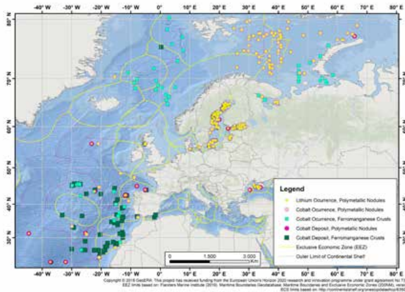
Figure 4: MINDeSEA pan-European map of energy-critical metals cobalt and lithium based on ferromanganese occurrences and deposits of nodules and crusts. Occurrences refer to \text{Li}_2\text{O} average content <660 g/t, potential resources <5,000 Mt, and Co average content <500 g/t. No up-to-date information is given about resource potential.
