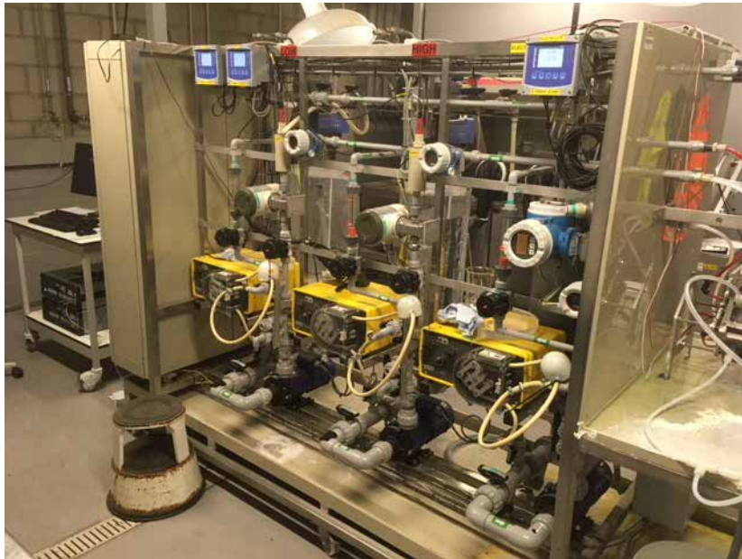
Figure 4: Semi-pilot setup for salt gradient power generation by reverse electro dialysis (SGP-RE) experiments (Photo: Joost Helsen)
