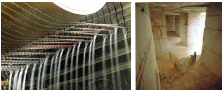
Figure 4: Innovation and technology: left - Multiwire block cutter (photo P. Primavori); right - underground marble mining (photo G. Milazzo).
