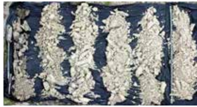
Figure 8: White bentonite from Spanish Lookout, Belize, the drilling core placed on plastic foil.
