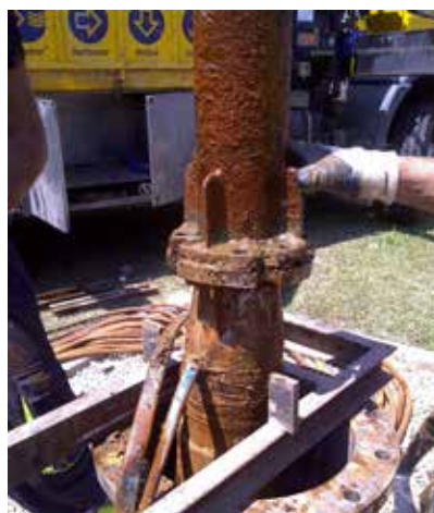
Figure 5. Well A, heavily incrustated rising main (left). Accumulation of fresh Iron precipitates on the rising main after a 12-hour pumping test (right).
