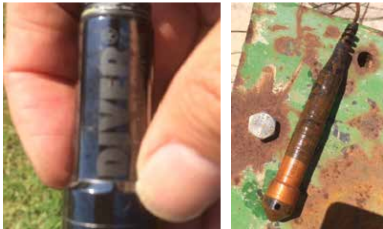
Figure 8: Comparison of fouling of dataloggers in an equalised well (Well A probe, left) and in a non-equalised well (Control well A', cable and probe, right) one year after installation.
