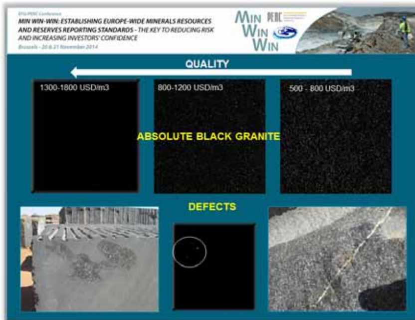
Figure 12: Example of defect in "Thaila Black" black granite currently quarried in Mauritania.
