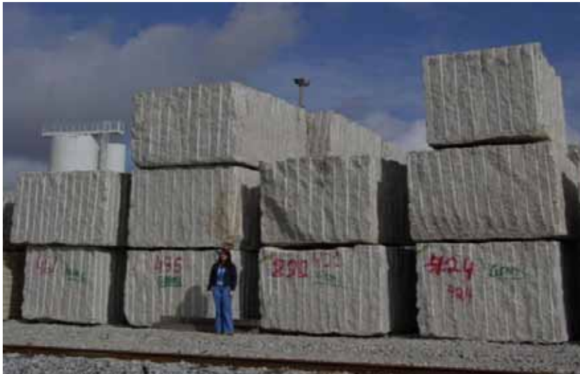
Figure 6: Regular large granite blocks, mined by drilling and splitting.
