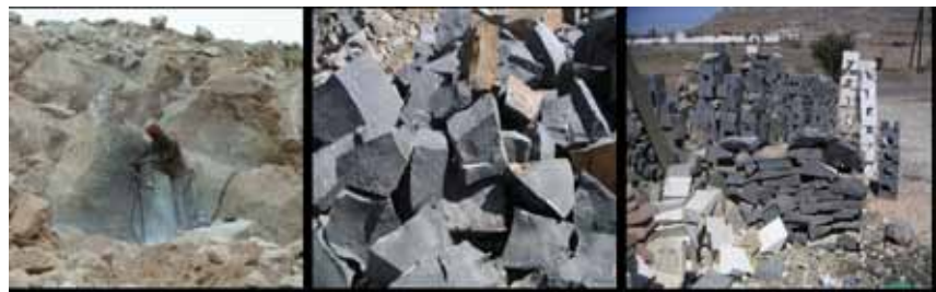
Figure 2: a. Typical quarrying methods for building stones - b. Building stones in small blocks - c. Building stones as final products (in this case, for cladding).
