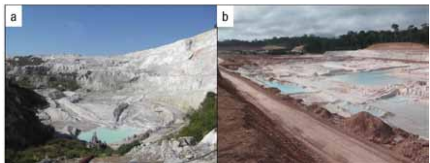
Figure 4: Photographs of (a) UK kaolin operations showing deep pits with centralised pond used to capture slurry washed directly at the face, and (b) Brazilian kaolin operations showing shallow, strip mining configuration, the photograph is taken from a reclaimed portion of the operation.
