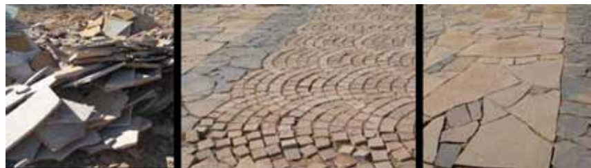
Figure 3: a. Naturally cleft stone (quartzite) slab - b. Ignimbrite cubes used for paving in the 'porfido' style - c. Quartzite paving slabs laid in style known colloquially as 'crazy paving'.
