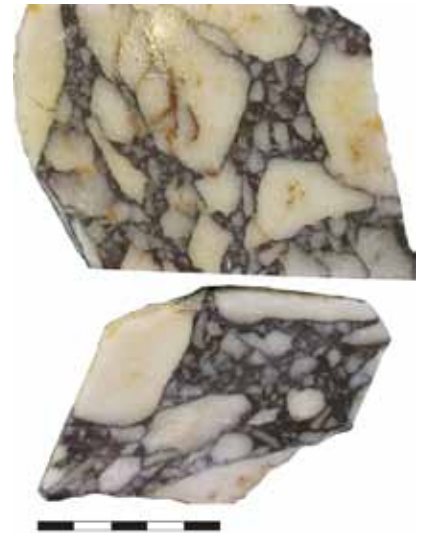
Figure 16: Slab of marble breccia with purplish matrix macroscopically assigned to the Marmo Pavonazzetto, probably originating from ancient Turkey. Basilica excavations, Tongeren. Collections of Agentschap Onroerend Erfgoed Brussels (Photo: R. Dreesen).
