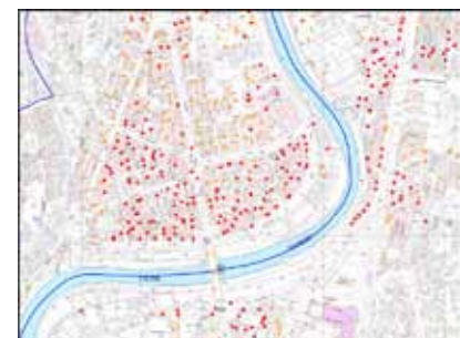
Figure 1B: Location of the project in relation to the evaluation of the maximum carrying capacity of the land, through the analysis of PSI points, highlighted by the movements of the adjacent buildings.
