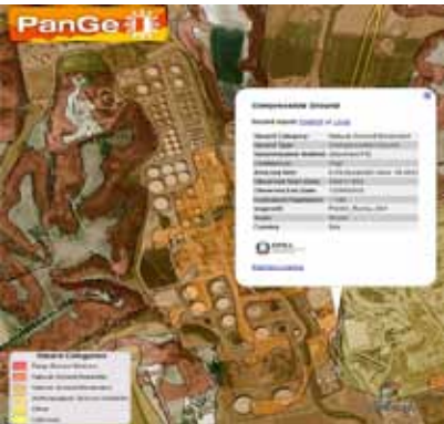
Figure 2C: Location of the project in relation to the Ground Stability Layer, which indicates compressible ground here.
