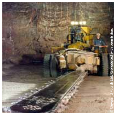
Figure 4: Undercutter in the Winsford salt mine (left) and an excavator in working in the Boulby Mine (right).
