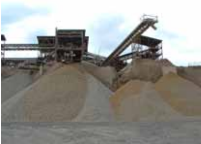
Figure 4: Dolostones aggregates preparation in the Marche-Les-Dames (Namur) quarry. (Goemaere et al., 2010).
