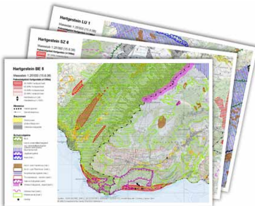
Figure 4: Potential maps show where, from a geologic point of view, potential high quality hard rock deposits are situated. The maps do not instruct about their suitability or economic viability. They further contain information about the relevant Federal or Cantonal inventories (e.g., ILNM), about building zones and partially about areas of water protection. They are suitable to reach a decision in the first planning steps, but are, however, not appropriate for detailed clarification.
