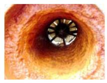
Figure 7: Iron oxide contamination, Tiwest Mine.
