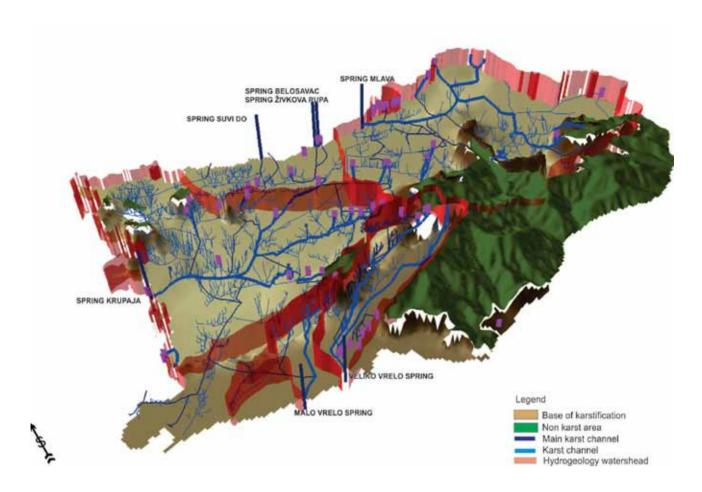
Figure 4: 3D model of karst channels in the Beljanica karst aquifer – a basis for a storage assessment and engineering regulation project (Milanović, 2010).
