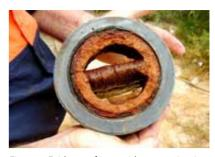
Figure 6: Evidence of iron oxide contamination, Tiwest Mine.
