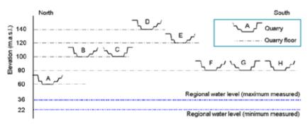
Figure 3: Unsaturated zone below the quarries.
