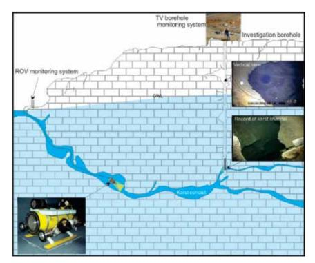
Figure 5: Research devices developed by CKH: cavities recorder ROV and logging video camera.
