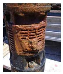
Figure 1: Iron oxide on pump removed from Lodi recharge well.
