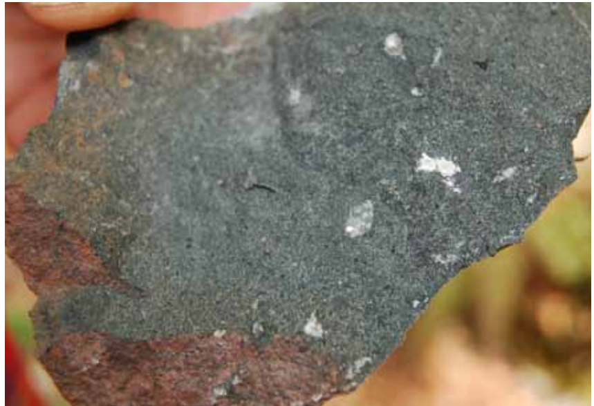
Figure 9: Almond-shaped geodes were formed in a diabase after the rapid cooling of lava flowing into the shallow sea in the Ladinian. White calcite crystals then filled the geodes. This almond-shaped diabase represents the western-most occurrence of magmatic rocks in Slovenia.
