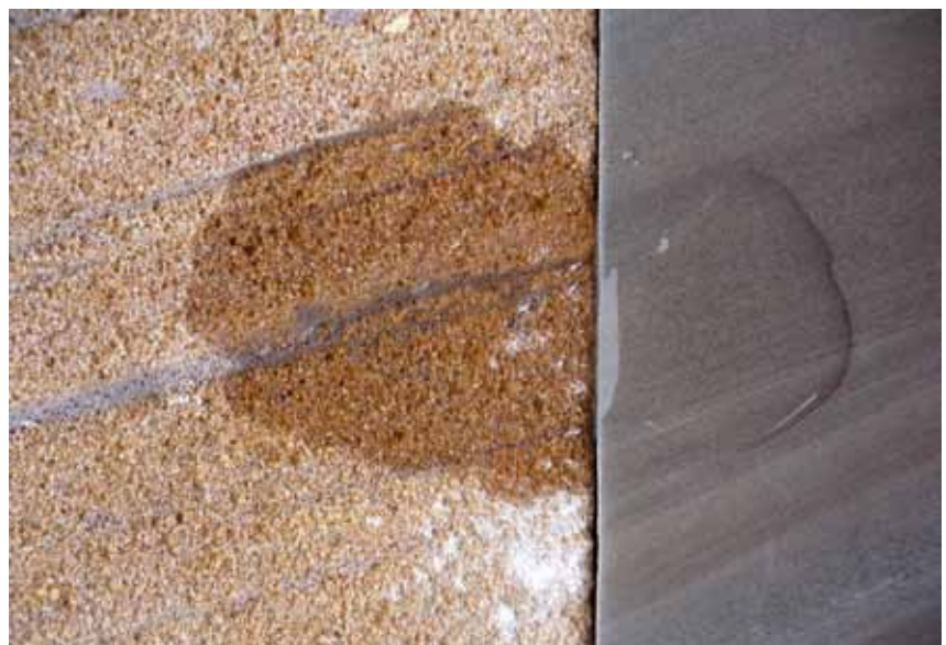
Figure 3: The result of a small test with water as an analogue to the behaviour of CO 2 at large depths. Water infiltrates rapidly into the porous sandstone (reservoir) on the left, but not into the impermeable siltstone on the right (reservoir seal).
