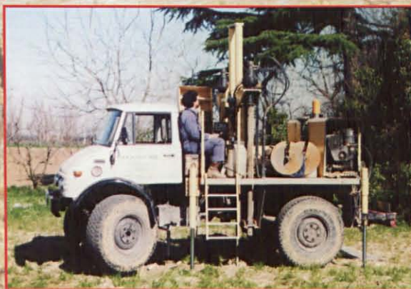
PENETROMETER TG 73-200 kN STATIC-DYNAMIC- ROTARY
