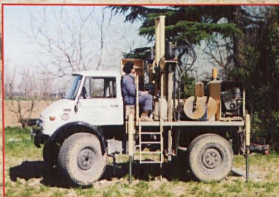
PENETROMETER TG 73-200 kN STATIC-DYNAMIC- ROTARY
