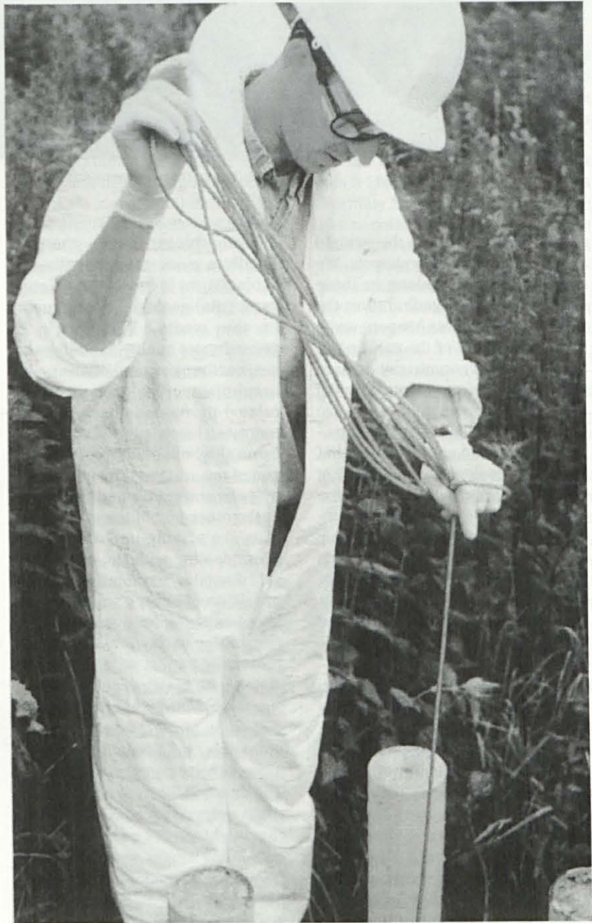
Sampling a monitoring well.
