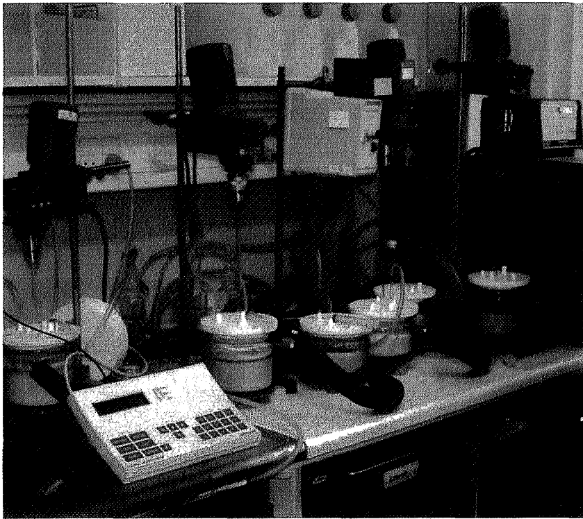
Figure 5. Experiments were conducted to determine the uptake mechanism of nickel by chalk. Results showed that nickel is not only adsorbed to the surface of calcite crystals but becomes incorporated.
