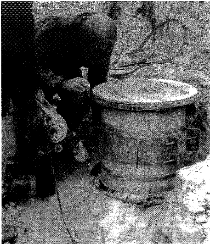
Figure 2. Columns 50 cm in length and diameter were drilled from the chalk and transported to the laboratory.
