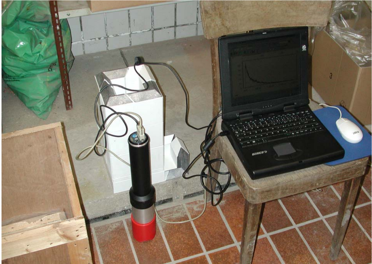
Figure 4.15: Gamma ray equipment; the detectortube (black) is connected with the sample holder (red) and the measurement takes place inside the Pb- shield (white).
