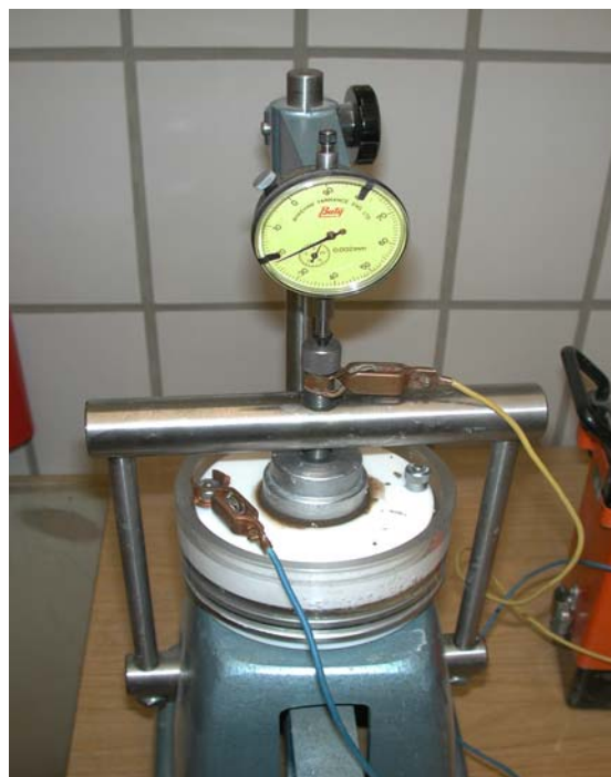
Figure 4.51: Measuring the resistivity during loading
