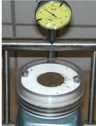
Figure 4.50: The oedometer with the sample in the ring of plastic
