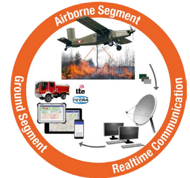
Figure 1: General concept of data acquisition, NRT communication and processing, data and resource management and information distribution to support time critical decision processes in forest fire situations
