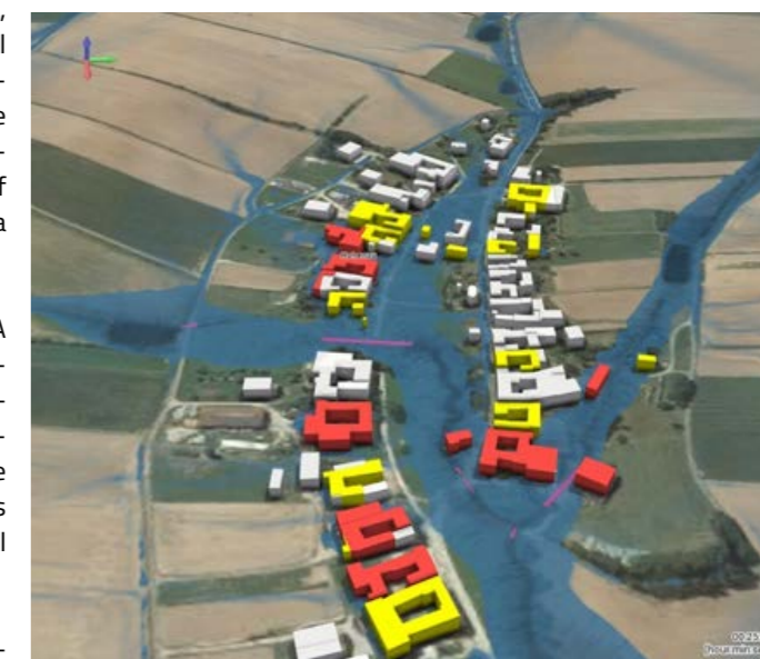
Figure 1: Example of pluvial flooding after 50mm of rainfall in 15 minutes; the building colour shows the maximum water depth: yellow = 50-100cm; red >100cm
