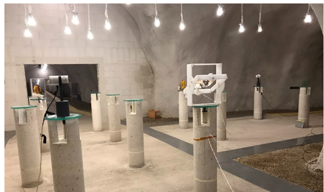
Figure 2: CSES-2 flight model sensor mounted on the (white) manual rotation frame in the absolute area of COBS.
