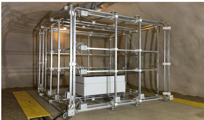
Figure 1: Three-meter Merritt coil system for magnetometer calibration in the calibration cavern of the Conrad Observatory.
