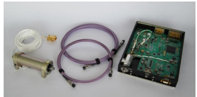
Figure 2: The flight model consists of a mixed signal electronics board and the laser unit mounted in the instrument box (right). The sensor unit (left) is located at the tip of a boom outside of the satellite and is connected with two fibres (middle) and the thermal control cable.
