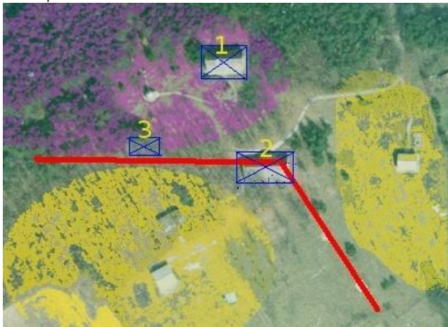
Figure 1: The picture shows the ground of Tihany observatory. The red lines are the fractures where the eruptions of hot water occurred. They separate the geological characteristics of the site i.e. rocky (purple) and clayey (yellow) areas. The blue rectangles are the places of geomagnetic measurements. 1 marks the absolute house, 2 marks the variation house and 3 marks a new underground hut.
