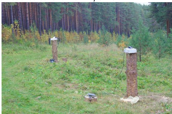
Figure 1: Intercomparison of scalar magnetometers GSM-19W (remote pillar) and POS-1 (near pillar). The supports were used to install the sensors in fixed place.
