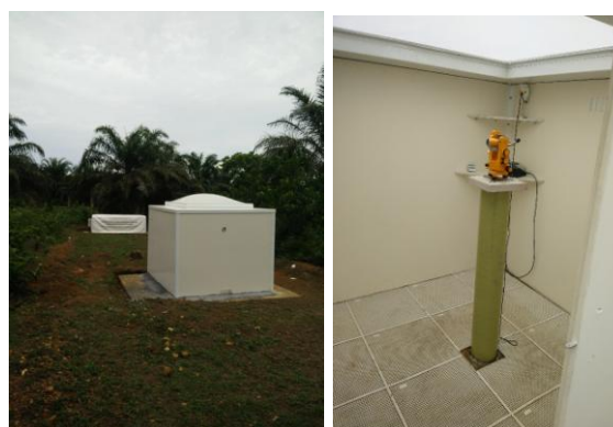
Figure 2: Left: picture of Edea observatory site showing the container with the sensors at the back and the absolute hut at the front. Right: picture of the absolute pillar in the absolute hut.
