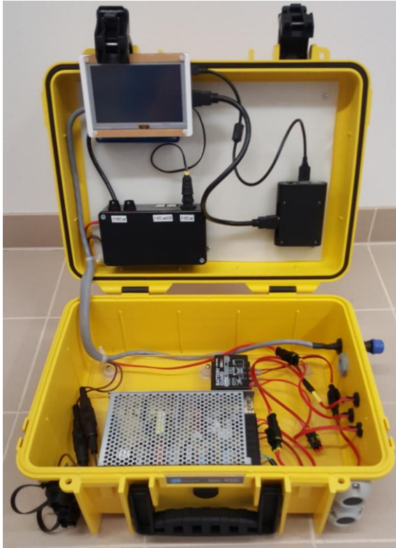
Figure 1: Connection box with mobile MARTAS system, unbreakable power supply (battery not shown), lightning protection, remote control.
