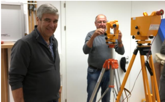
Figure 1: Test of a steel-free converted Zeiss THEO 020A theodolite during the IAGA Workshop 2018. From left to right: Alan Berarducci, Jörg Krüger, Theo 020A, Carl Zeiss Jena Ni 002 collimator with green light source at ocular.
