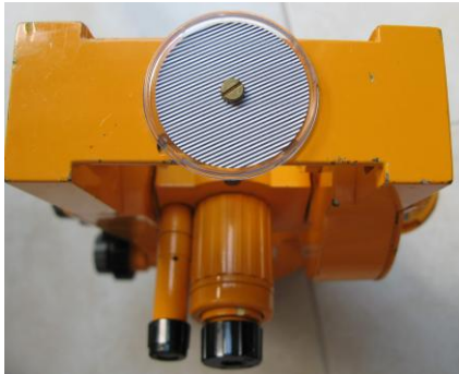
Figure 1: Multi-parallel line pattern fixed on the top of a Zeiss theodolite
