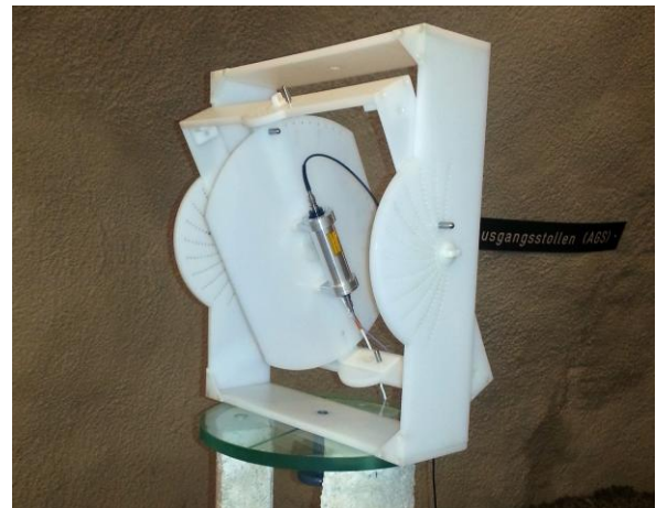
Figure 3: The CDSM sensor unit is mounted on the rotation device on a pillar of the Conrad Observatory. Measurements are compared to an Overhauser reference magnetometer on another pillar.
