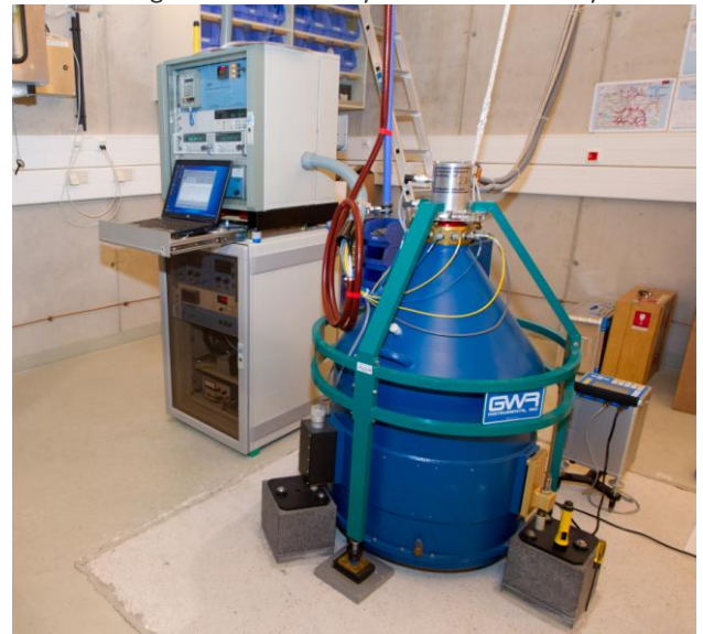
Figure 2: The gravimeter at the Conrad Observatory
