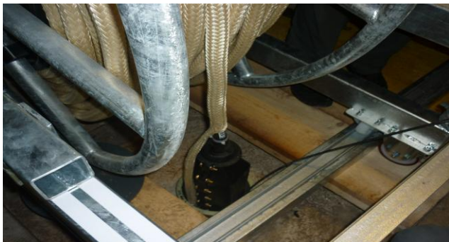
Figure 1: The sensor electronics, which finally remains in a distance of 7 m above the supergradiometer sensor, is lowered into the bore hole.
