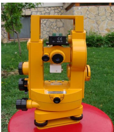
Figure 1: D/I theodolite with FLUXSET.
