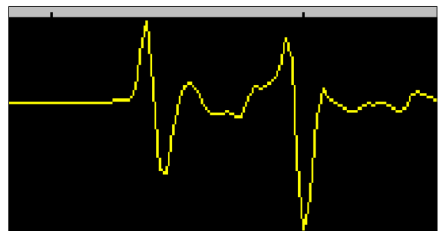
Figure 3: N-shaped signal of a supersonic aircraft.
