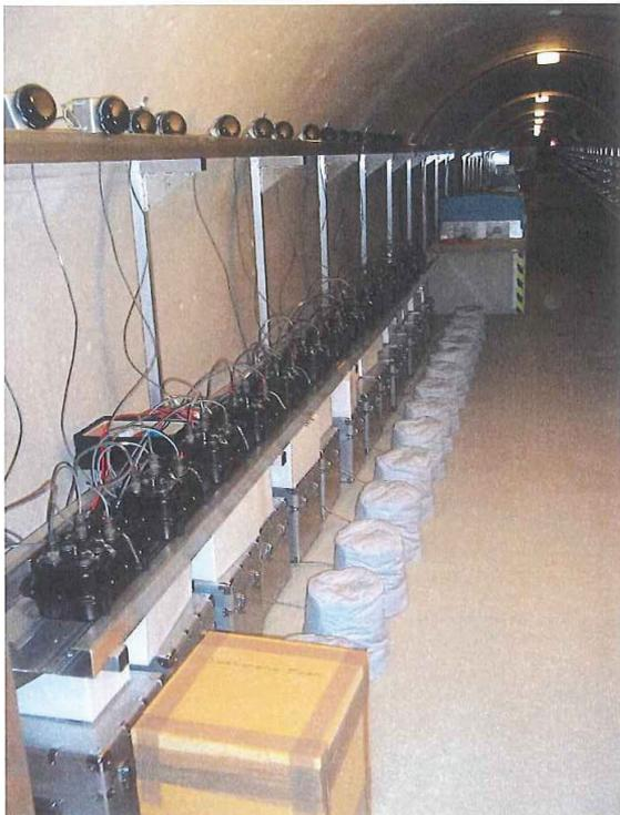
**Figure 1:** 15 broadband sensors, recorders, and GPS antenna in the tunnel of the Conrad Observatory.
