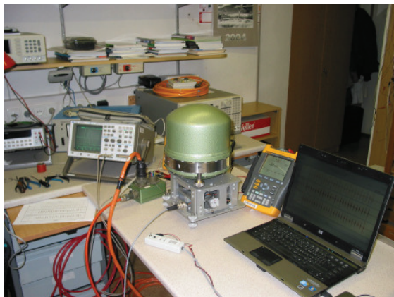
Figure 1: Calibration Table CT-EW1 in the Institute of Physics of the Earth, Brno with STS-2 seismometer.
