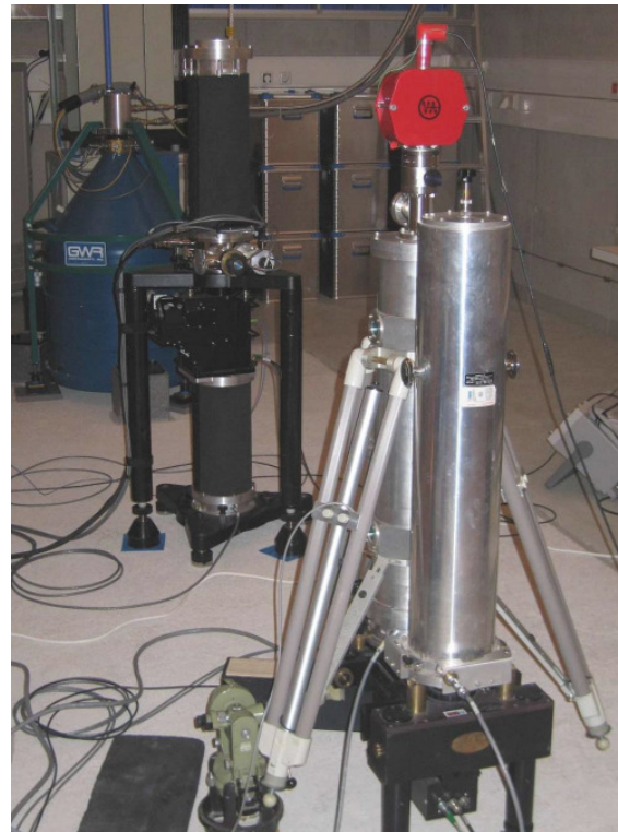
Figure 2: Absolute gravity measurement survey for SG calibration (FG5, front: JILAG-6)
