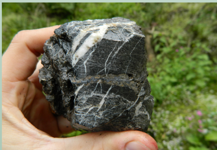
Base metal minerals such as galena and sphalerite in vein on picture, can be carriers of several trace elements categorised as CRM (Ga, Ge and In for instance), which increase the value of the deposit.
