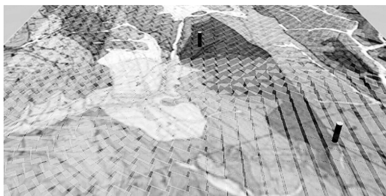
Fig. 3. Spatial distribution of fractures in Nowa Ruda serpentinite massif (SW Poland) – view 2.
