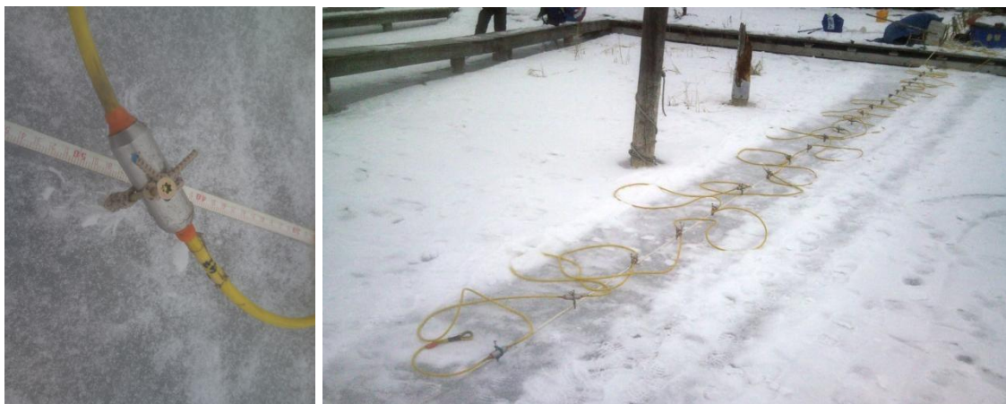
Fig. 15.7: Layout of the geoelectrical line on the ice cover of lake Neusiedl (right); coupling of cables to the ice sheet using screws
