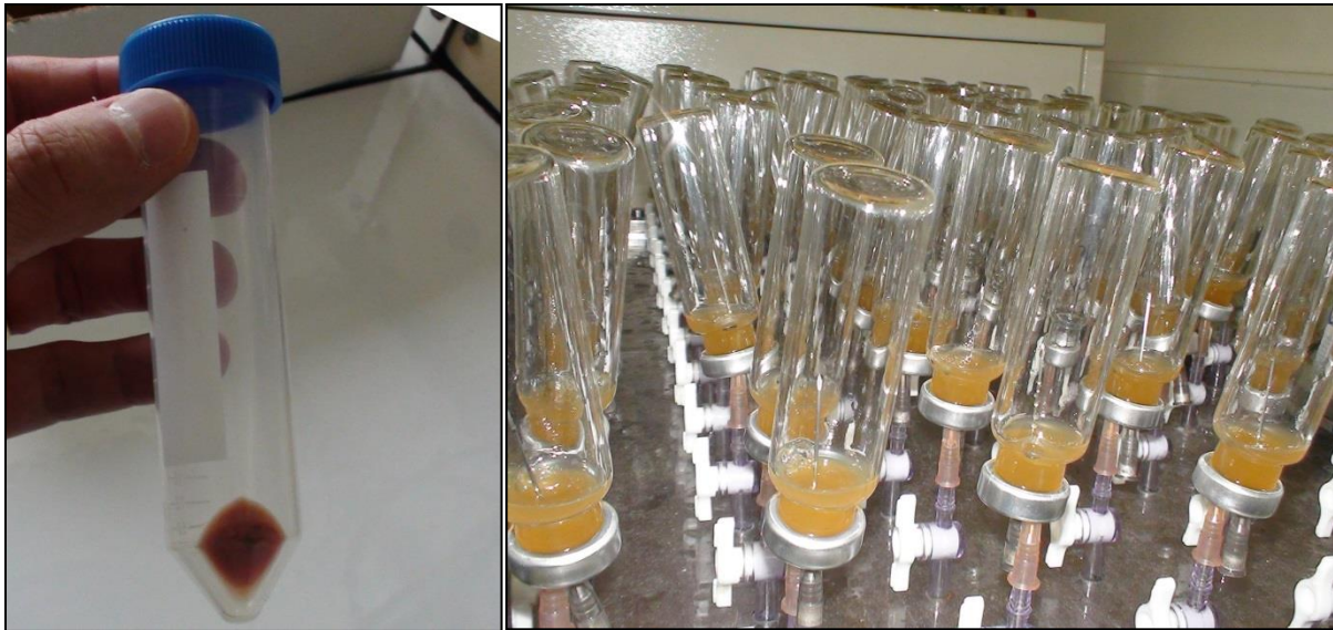
Figure 2: Left: Isolated Pseudomonas aureofaciens bacterial; Right: Helium injection for degasification of the vials.
