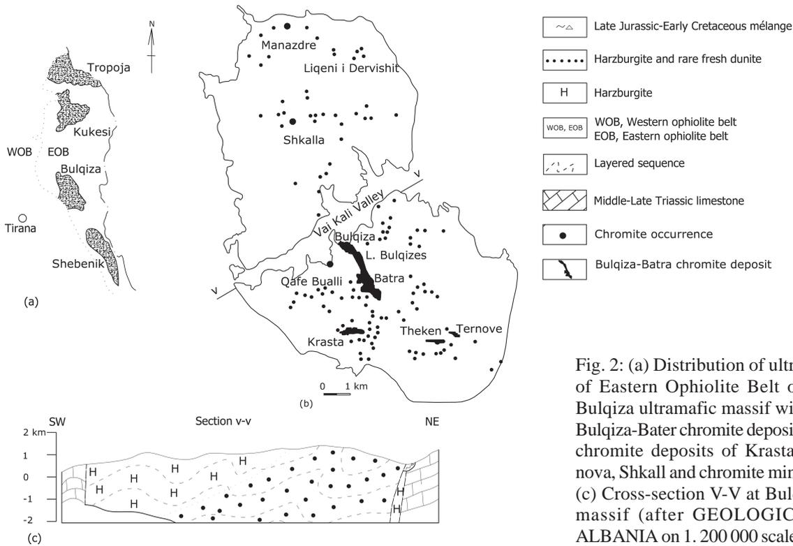
Fig. 2: (a) Distribution of ultramafic massifs of Eastern Ophiolite Belt of Albania. (b) Bulqiza ultramafic massif with plan view of Bulqiza-Bater chromite deposit and other main chromite deposits of Krasta, Theken, Ternova, Shkalla and chromite minor occurrences. (c) Cross-section V-V at Bulqiza ultramafic massif (after GEOLOGICAL MAP OF ALBANIA on 1: 200 000 scale 1983).
