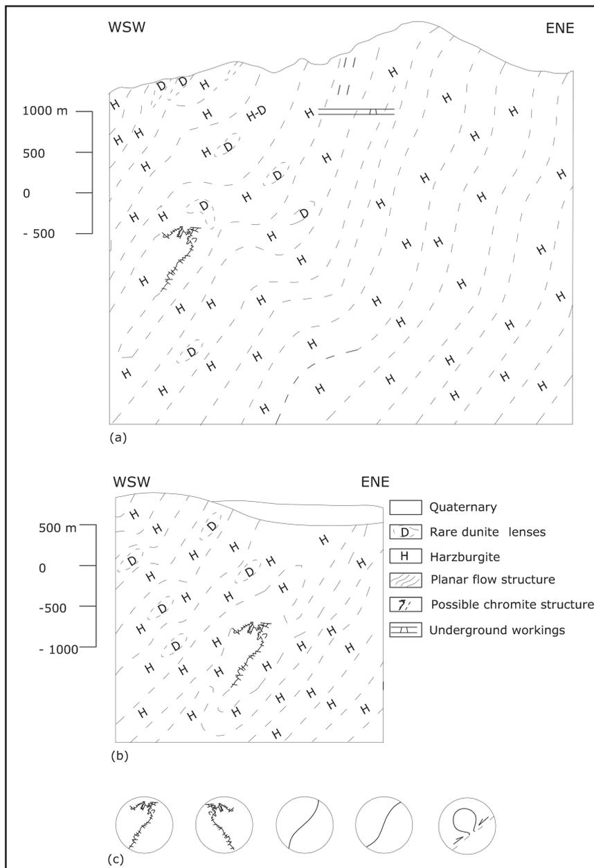
Fig. 5: (a) Vertical WSW-ENE cross-section -193 at northern part of Bulqiza massif with possible chromite structure. (b) Vertical WSW-ENE cross-section -59 at northern part of Bulqiza massif with possible chromite structure. (c) Possible fold displays of chromite layer as result of deformation.
