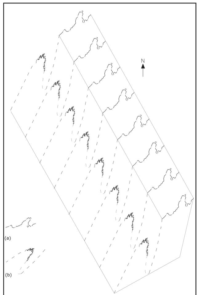
Fig. 7: 3D representation of Bulqiza chromite ore structure: (a) the chromite mineralization is supposed to be developed as eastward overturned gentle folding (see Fig. 6a) whereas at (b) the chromite structure presents an eastward overturned antiform with limbs developed in vertical plane. Note the change with a horizontal angle of almost 90° between two views.
