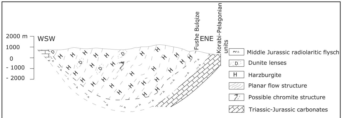
Fig. 8: Generalized vertical WSW-ENE cross-section of Bulqiza ultramafic massif showing location of Bulqiza eastward overturned chromite antiform in conformity with planar flow structures of the homocline massif.
