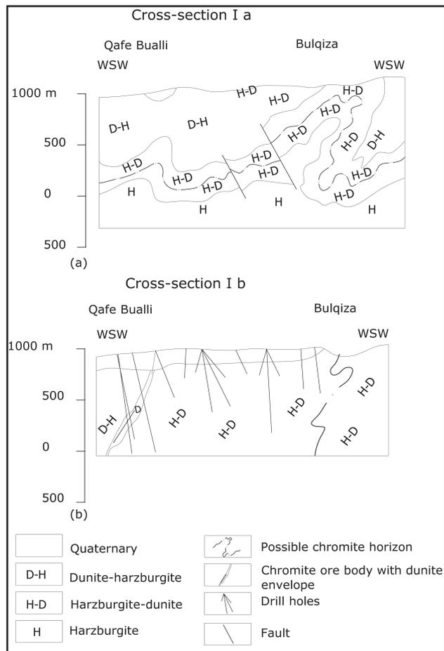
Fig. 6: Vertical WSW-ENE cross-section Ia, Bulqiza-Qafe Bualli deposit, showing possible chromite structure (after QORLAZE et al. 1989). Vertical WSW-ENE Cross-section Ib Bulqiza-Qafe Bualli deposit, showing the results of drill holes between Bulqiza and Qafe Bualli and a tabular chromite ore body encountered by drill holes at Qafe Bualli.
