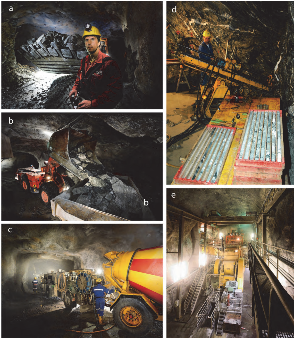
Fig. 20: a. Remote-controlled scooptram with 15 tonnes capacity. b. Mucking into an ADT truck for underground haulage from the lower sublevels. c. Shotcreting of development drifts. d. Underground diamond drilling. e. Primary jaw crusher in the underground crushing station.
