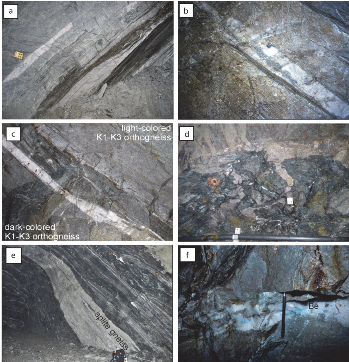
Fig. 11: a. Well-foliated K1-K3 orthogneiss with deformed quartz vein (Quartz 1) and rafts of strongly deformed hornblende-biotite schists. K1' ore body, level 1164; photo J.G. Raith, February 2009. b. ≈10 cm thick deformed quartz vein containing elongate scheelite (grey, Scheelite 2) in K1-K3 orthogneiss. The mineralised vein crosscuts the Early Carboniferous granite gneiss (336-341 Ma, Kozlik et al., 2016b) but shows penetrative deformation. Upper part of K1 orebody, level 1152; photo J.G. Raith, September 1999. c. Sharp contact between dark- and light-coloured K1-K3 orthogneiss varieties. A quartz-scheelite vein (white) crosscuts the gneiss but is aligned in the foliation; level 1164; photo M. Kozlik, 2013. d. Folded apophyses of dark-coloured K1-K3 orthogneiss intruding amphibolite; level 1164 m; photo J.G. Raith, February 2013; rectangular scale length ≈8 cm. e. Dike of aplite gneiss aligned in dark foliated fine-grained amphibolite; dyke is about 1 m thick; level 940; photo M. Kozlik, 2013. f. Quartz-scheelite vein with beryl (Be) crosscutting K1-K3 orthogneiss; level 1164; pen for scale is 12 cm; photo M. Kozlik, 2013.
