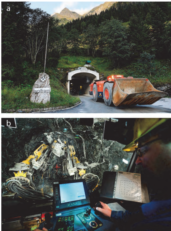
Fig. 19: a. Portal of the Felbertal underground mine. b. Drilling with modern computer-controlled two-boom jumbo.
