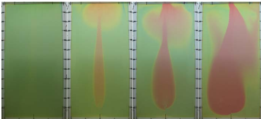
Fig. 3: Representative photos for CO 2 gas injection and application of resistivity tomography survey.
