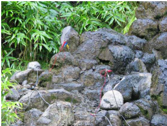
Fig. 7: Electrodes used for monitoring of geyser.
