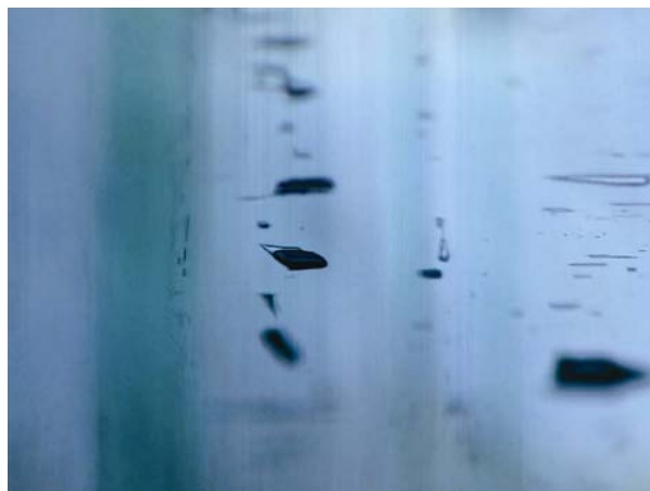
Fig. 2. Enlarged area of the photomicrograph of primary fluid inclusions Figure 1 showing alternating coloured and clear areas in the zoned emerald crystal. The clear zones correspond to growth zones dominated by primary vapour rich fluid inclusions.
