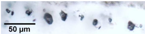
Fig. 3. Coexisting liquid-rich and vapor-rich inclusions in an FIA from the shallow, high-oxidation part of the system (100 m present day depth).
