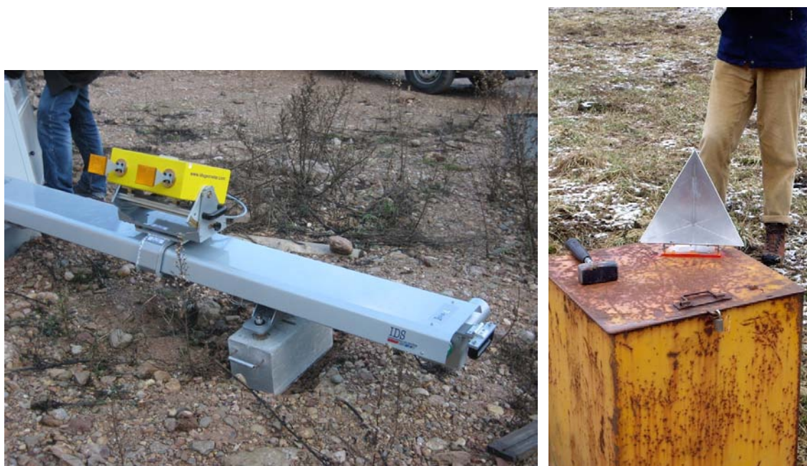
Fig. 3: The IBIS-L-IDS GBSAR system installed in front of the Vallcebre landslide by the Institute of Geomatics for the first tests. A number of mini-corners (right) were deployed in the scene.
