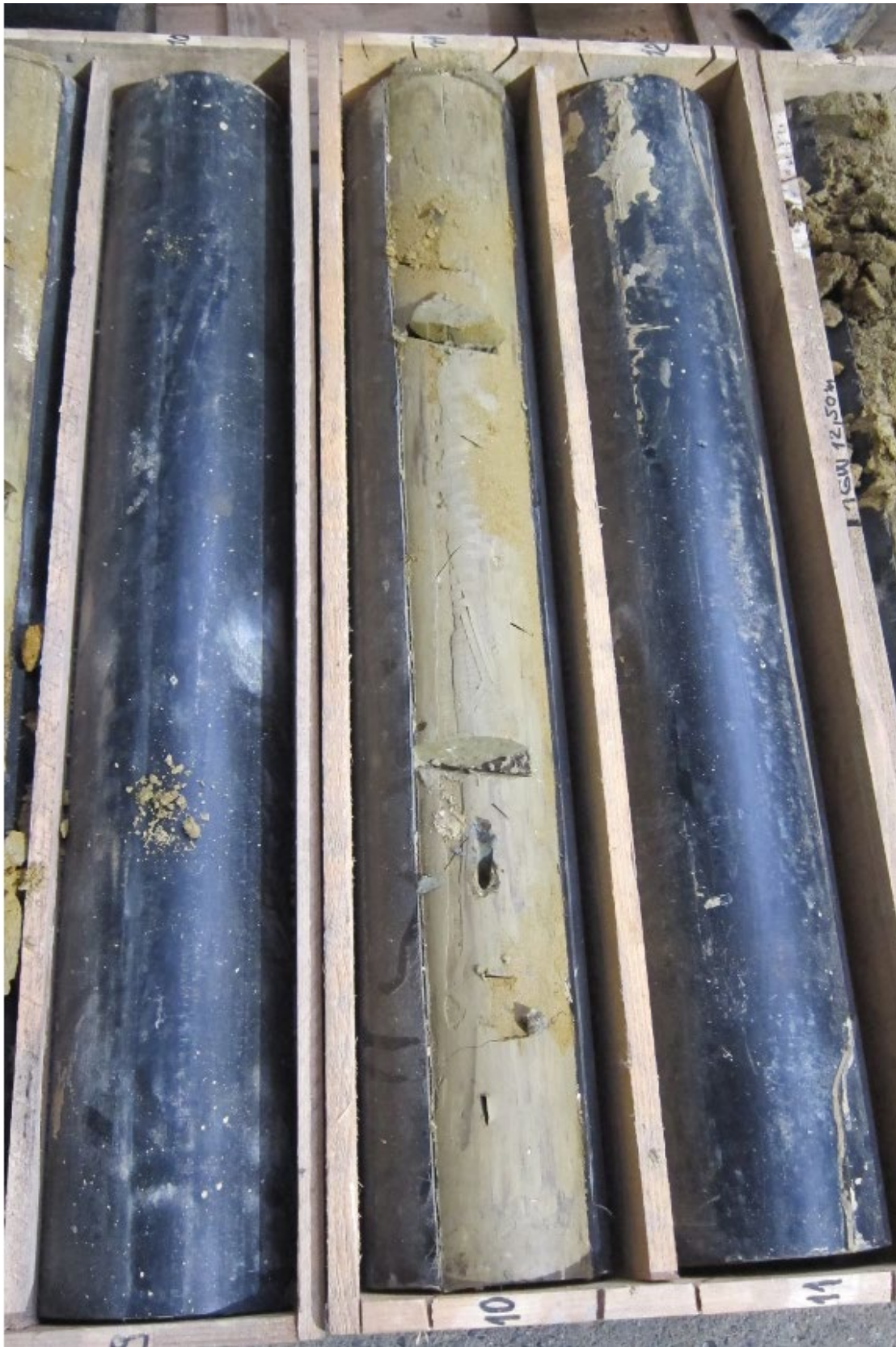
Abb. 2.1.1.30.: Bohrkerndokumentation KB17 (9,0-12,0m) (Foto: M. Peresson).
