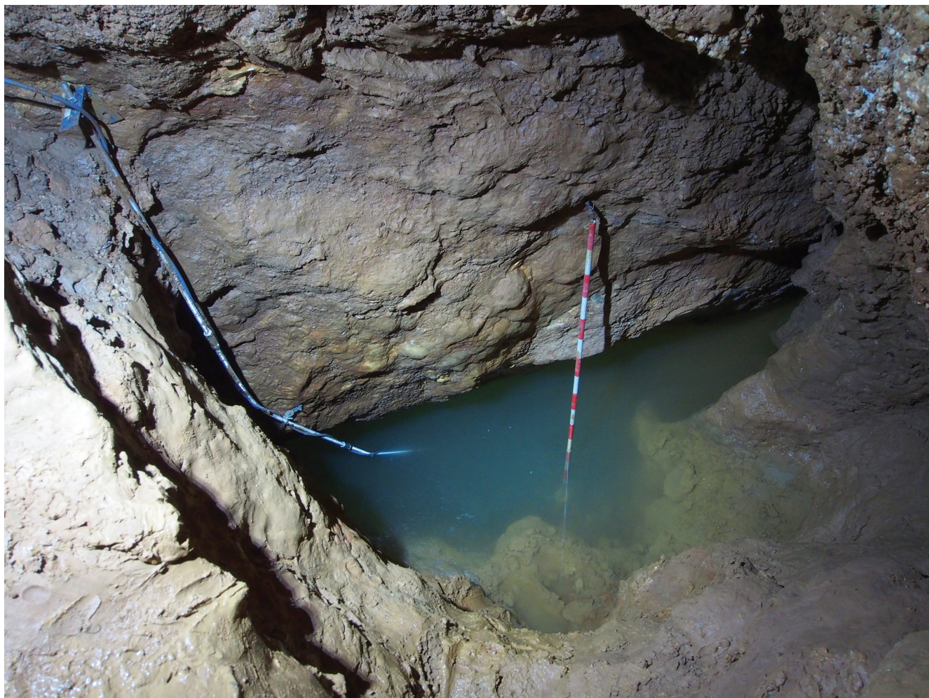
Figure 4: Thermally influenced spring with stick gauge and data logger.
